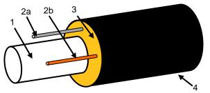
Figure 1. Schematic view of the end of a district heating pipe where a joint has to be made. (1) Service pipe (steel), (2) Leak detection ((2a) tinned copper, (2b) copper), (3) Insulation (PUR) and (4) Casing (PE).
