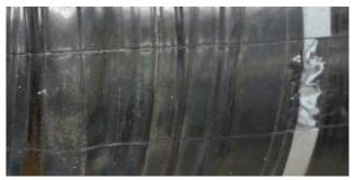
Figure 12. These tapes were strongly bonded to the PE casing. The edge on the right side shows unsuccessful attempts to detach the tape.
