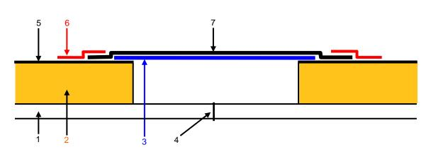
Figure 2. Cross-section of a joint (schematic). (1) Service pipe (steel), (2) Insulation (PUR), (3) Optional shrink film, (4) Weld in the steel pipe, (5) Casing (PE), (6) Shrink collar (PEX) or tapes (butyl rubber, Densolen N8 and black Denso foil) and (7) Shrink sleeve (PEX or PE) or welded sleeve (PE).
