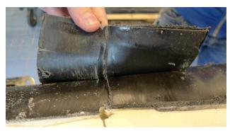
Figure 13. The collar of this PEX shrink joint could easily be detached manually from the casing and the PEX shrink sleeve.
