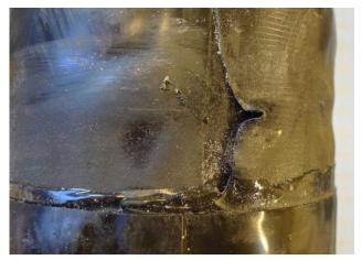
Figure 5. Fold in PEX shrink sleeve.
