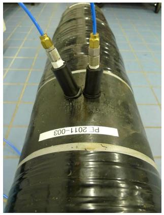
Figure 3. Connections to a district heating pipe joint using two hollow PE rods to perform the leak tightness test.
