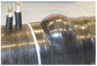
Figure 10. Failed joint after being pressurised up to 1.5 bar(g).
