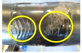
Figure 6. Wrinkles in the collar of a PEX shrink sleeve.
