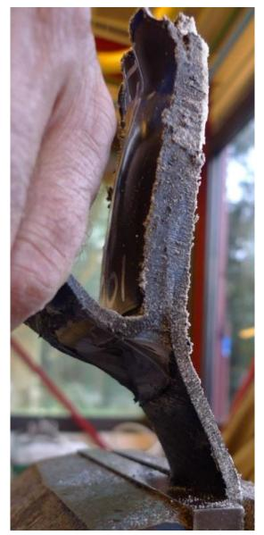
Figure 16. The bonding between the PEX shrink sleeve and the PE casing is strong enough to withstand manual peeling.
