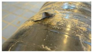
Figure 7. A tape ending halfway across the taped area. This causes a weak spot in the system.
