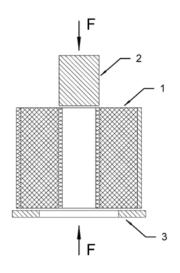
Legend 1 test specimen 2 piston for load impact F 3 support
