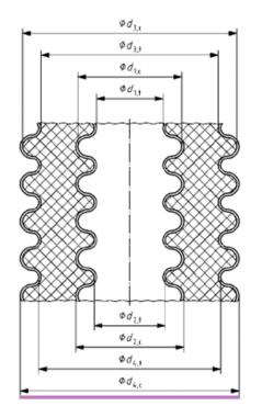
Figure II.2: diameters of corrugated pipe
