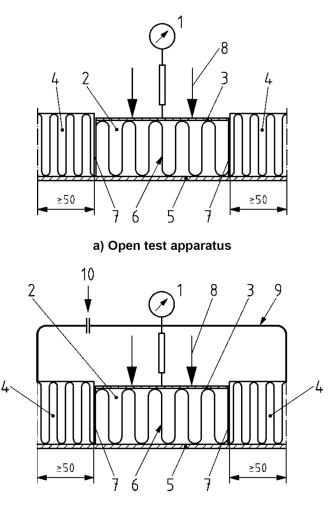
b) Test apparatus with cover gas
